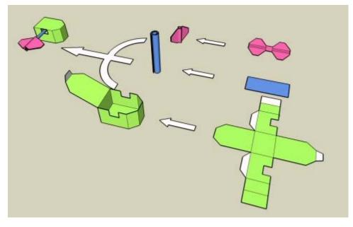
assemble the parts into a neck
